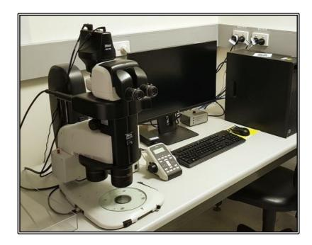
Available Objective Lenses: 0.5x and 1.0x lens plus Magnification Range of 0.75 – 13.5x
