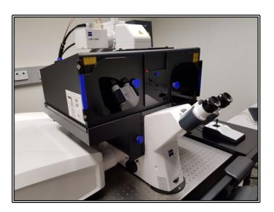
**Available Objective Lenses**: 10x Air, 20x Air, 40x Oil and 63x Oil (40x Water is also available) **Available Laser Lines**: 405, 458, 488, 514, 561 and 633nm
