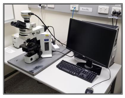
Available Objective Lenses: 2x Air, 10x Air, 20x Air, 40x Oil, 60x Oil and 100x Oil
