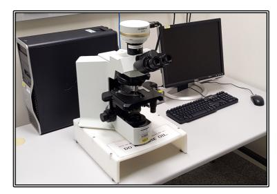
Available Objective Lenses: 2x Air, 4x Air, 10x Air, 20x Air, 40x Air
