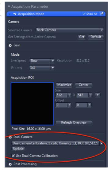
• If Image Alignment is required, select the Dual Camera Calibration Wizard from the Acquisition menu at the top of the screen.
