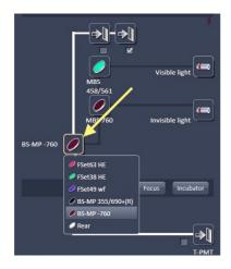
• Select one or both of the NDD channels. These have fixed bandpass filters covering the emission ranges 500-550 and 575-610nm, respectively.
