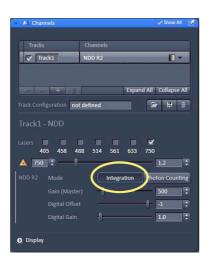
**Warning**: The non-descanned detectors are extremely sensitive and easily damaged by excess light. Start with **LOW** laser powers and detector gain settings.
