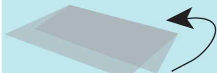
3. Wipe the folded lens tissue across the front of the objective lightly once more to remove any excess immersion fluid
